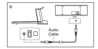
C. Plug one end of the audio cable into the jack on the front of the Incline Trainer near the power cord. Plug the other end of the cable into a 3.5mm Y-adapter (available at electronics stores). Plug the Y-adapter into the PHONES jack on your stereo. Plug your headphones into the other side of the Y-adapter.
